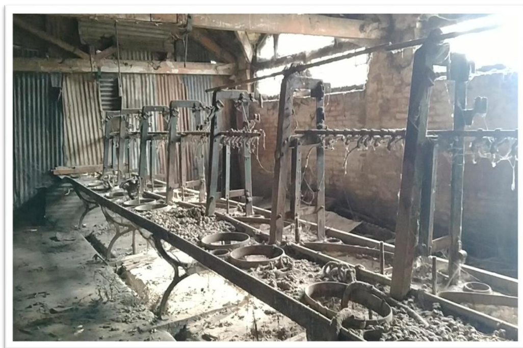
Figure 5: Cottage basin reeling machine in a dilapidated silk filature established in 1917 at Solina, Srinagar, Jammu and Kashmir.
