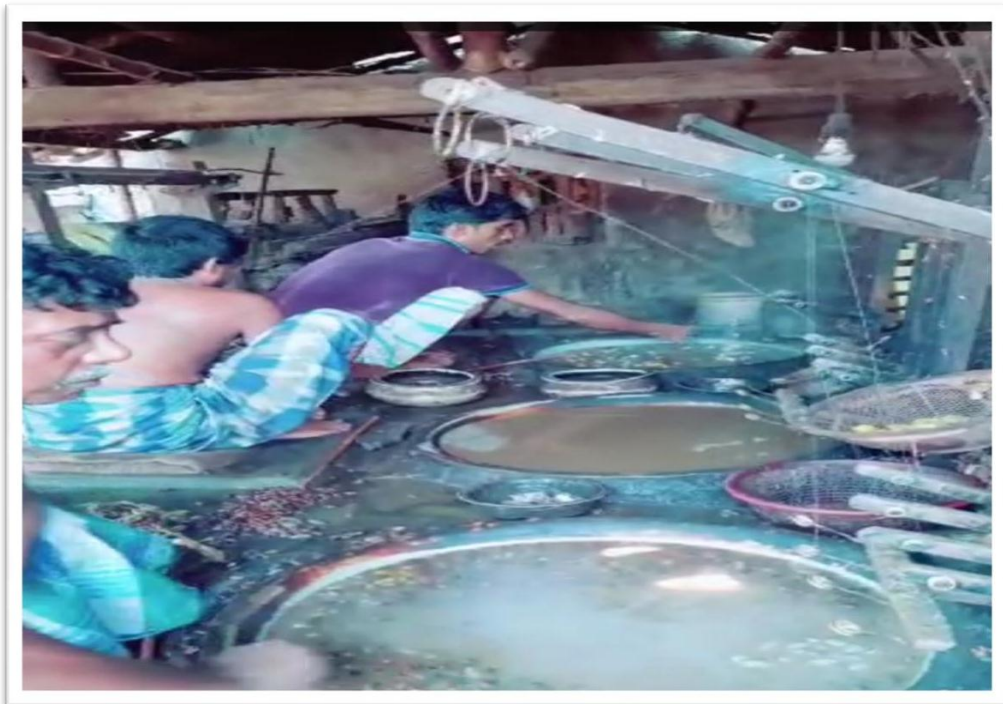
Figure 4: Reeling done on country charkha by a reeler
